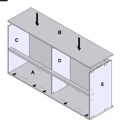
Select centre set of holes and bore holes through base and top panels as shown.
