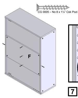
Screw fix through base and top panel into top and bottom edges of rear support panel F.
