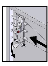
Insert left and right hand adjustable wall brackets into holes at rear of unit. Lock in place with rear lock clips and secure each bracket with screws as shown.
