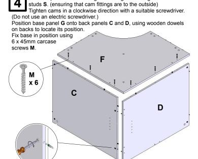
Fix back panels C and D together using cam fittings K and cam
