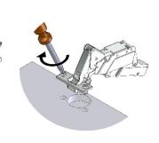
Clip hinges onto hinge plates. To release hinges from plates, lift the rear release clip as shown.
