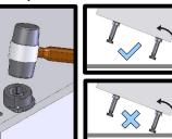
Fit the leg bosses into the base panel of the unit. Turn the leg boss so the flange
