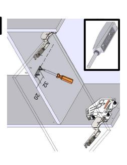
13 On 'Touch' open units a push open catch should be fitted in the centre of the mid shelf as shown.
