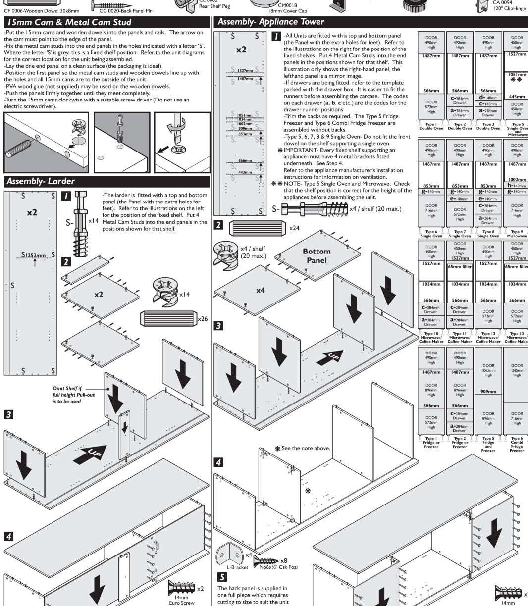
ordered. The Type 5 and Type 6 Fridge Freezer housings are assembled without a back.
